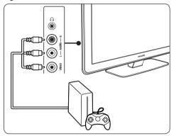
A permanent game console or camcorder can be connected to a HDMI connector or EXT 3 (component) connectors at the back of the TV.
