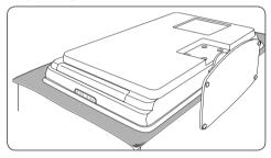
2. Using a cross-head screwdriver (not supplied), unscrew the four bolts that secure the stand to the TV.
