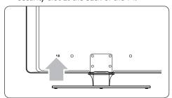
If connecting an anti-theft Kensington lock (not supplied), position the TV within reach of a permanent object (such as a table) that can be easily attached to the lock.
