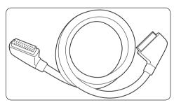
SCART combines audio and video signals in one cable. Audio signals are stereo, while video signals can be composite or S-Video quality. SCART does not support high-definition video and is analogue. Two SCART connectors are provided on the TV, EXT 1 and EXT 2.
