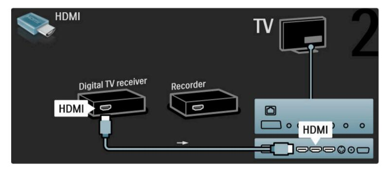
Finally, use an HDMI cable to connect the Disc Recorder to the TV.
