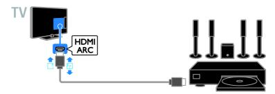
Connect the home theatre with an HDMI cable and an optical audio cable to the TV.
