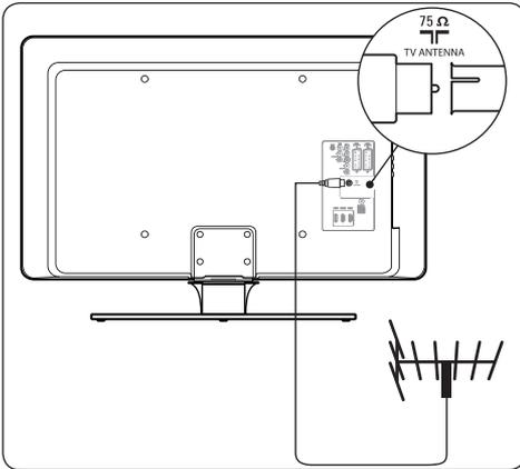
1. Locate the **TV ANTENNA** connector at the back of the TV.
