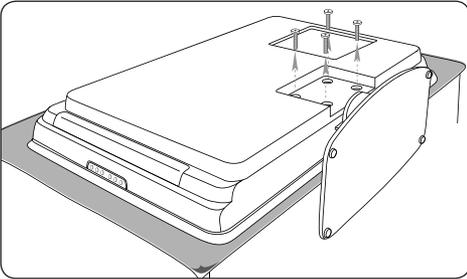
3. Firmly pull the stand from the bottom of the TV. Place both the stand and bolts in a secure location for future reinstallation.
