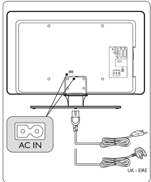
1. Locate the **AC IN** mains connector at the back or on the bottom of the TV.
