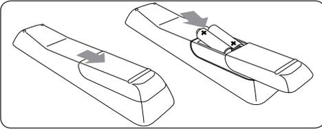
1. Slide the battery cover off the back of the remote control.
