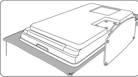
2. Using a cross-head screwdriver (not supplied), unscrew the four bolts that secure the stand to the TV.
