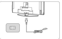
The TV is never powered off completely unless the mains cord is physically unplugged. Therefore the mains plug must be accessible at all time.
