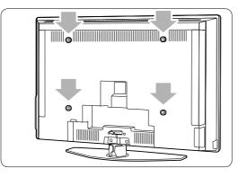
2 Unscrew the discs and use the free holes (M8) for fixing the VESA wall bracket.
