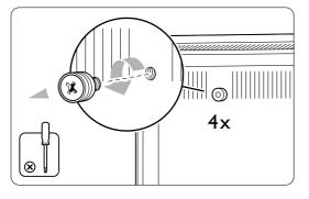
**3** To remove the TV stand locate the 4 screws of the TV stand.
