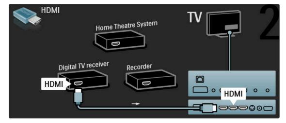
Then use an HDMI cable to connect the Disc Recorder to the  ${\sf TV}$ .
