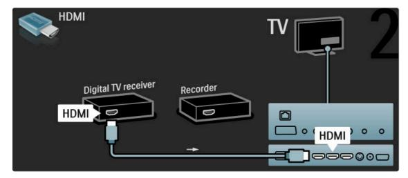
Finally, use an HDMI cable to connect the Disc Recorder to the  ${\sf TV}$ .
