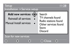
The search begins and only new channels will be stored and added to the channel list menu. The percentage of the installation that has been completed and the number of channels found is displayed. When the search is completed, press the OK key to accept the new services.
