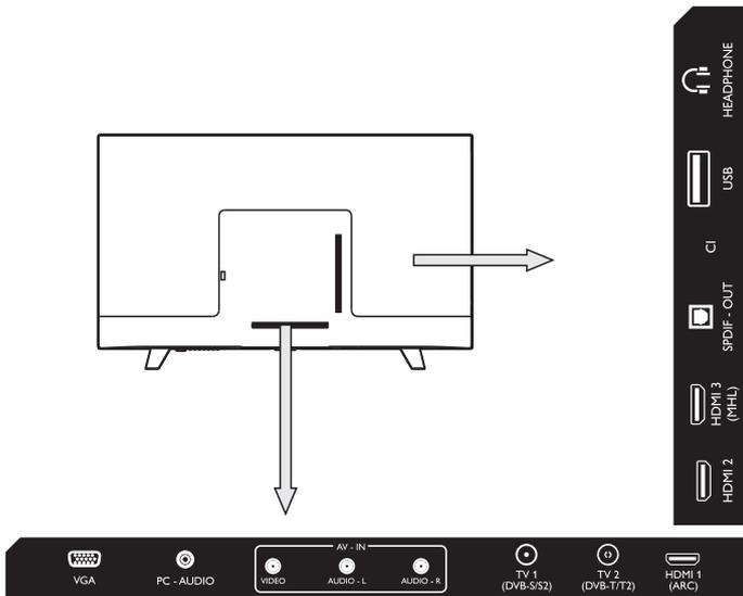
Always connect a device to the TV with the highest quality connection Available. Also use good quality cables to ensure a good transfer of picture and sound. If you need help to connect several devices to the TV, you can visit the Philips TV connectivity guide. The guide offers information on how to connect and which cables to use. Go to [www.connectivityguide.philips.com](http://www.connectivityguide.philips.com).
