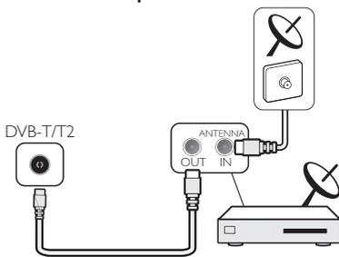
If you have a Set-top box (a digital receiver) or Recorder, connect the antenna cables to run the antenna signal through the Set-top box or Recorder first before it enters the TV. In this way, the antenna and Set-top box can send possible additional channels to the Recorder to record.
