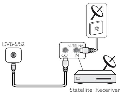
Connect the dish antenna cable to the satellite receiver.
