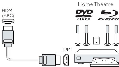
Use an HDMI cable to connect a Home Theatre System (HTS) to the TV. You can connect a Philips Soundbar or an HTS with a built-in disc player.
