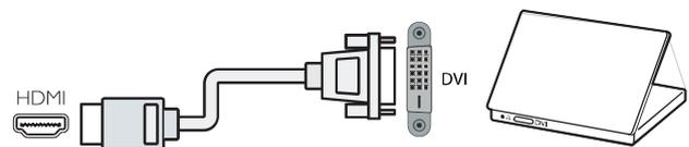
If you still own a device that only has a DVI connection, you can connect the device to any of the HDMI connection with a DVI to HDMI adapter.
