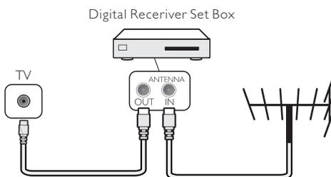
Use 2 antenna to connect the antenna to the Set-top box (a digital receiver) and the TV.
