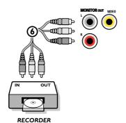
The **MONITOR OUT** connector can be used for daisy chaining or to record programs from your TV (6). Only when a recorder is connected to **MONITOR OUT** it is possible to record an analog program from your TV. See Record with your recorder, p. 13.
