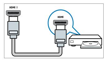
Connections via DVI or VGA require an additional audio cable (see 'Connect a computer' on page 27).
