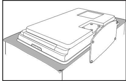
4. Using a cross-head screwdriver (not supplied), unscrew the four screws that secure the stand to the TV.
