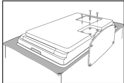
5. Firmly pull the stand from the bottom of the TV. Place both the stand and screws in a secure location for future reinstallation.
