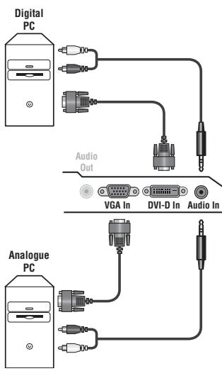
Connect the monitor output of your computer to the **PC VGA In** or **DVI-D In** of the TV.
