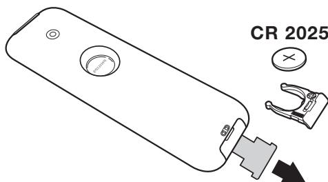
Pull out the plastic insulation sheet from the battery to activate the remote control.
