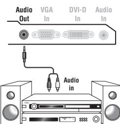
To connect to a home theater or hi-fi system, use an audio connection cable and connect the sound output **Audio out** on the TV set to the "AUDIO IN" "L" and "R" input on your hi-fi amplifier.
