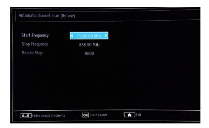
Press "OK" to start the installation process. During this progress the bar will fill and found channels will be added to the list.
