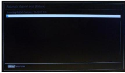
Note: If option Aerial & Cable option is selected, when DVB-T channel search is complete, you need to define the start frequency, end frequency and step for DVB-C channels. If you don't know those values, use the default ones and press "OK" to start the search.
