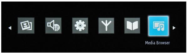
You can play photo, music, and movie files stored on a USB disk by connecting it to your TV. Connect a USB drive to one of the USB inputs located on the side of the TV. TV will read the content and provide an option to browse the USB drive. In Media Browser setting the following items are available: Videos, Photos, Music and Settings.
