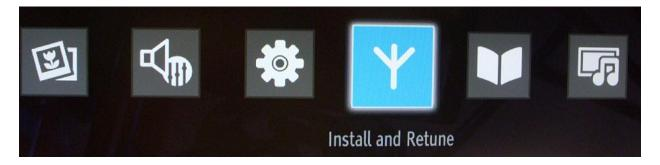
The menu contains options for automatic channel install, manual channel install, network scan, analog fine tune for a better reception of the analog TV channels. The first time installation option will delete the TV channels and set all settings to default values, except Hotel TV settings.
