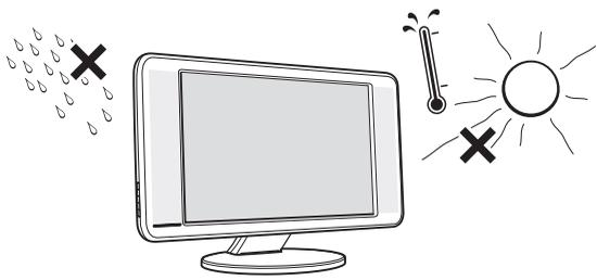
Place your LCD TV on a solid stable surface that can support the LCD TV weight.
