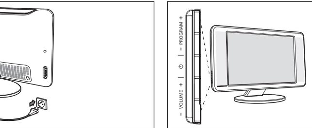
2) Connect the mains cord to the television power inlet and the mains plug to the wall socket.
