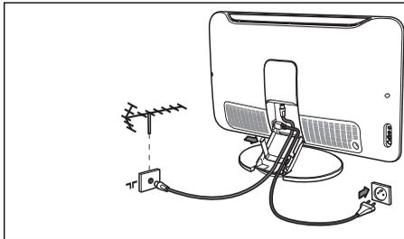
1) Use the aerial connection lead supplied to connect the aerial socket of the TV to the **T** socket.
