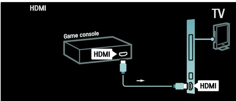
If you cannot use the side connector, use an HDMI or the EXT2 (YPbPr and Audio L/R) cable to connect the game console to the back of the TV. (On certain models, EXT2 is labelled EXT3).
