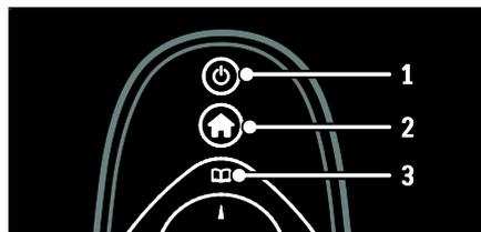
1. **Power (Standby)** : Switches the TV to standby if it is on. Switches on the TV if it is in standby.
