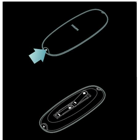
For remote control with AAA batteries (side by side):
