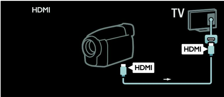
Otherwise, use an HDMI cable or the component video and audio cable (YPbPr and Audio L/R) to connect the camcorder to the back of the TV.
