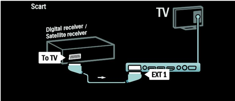
Finally, use two SCART cables to connect the two devices and the TV.
