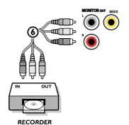
The **MONITOR OUT** connector can be used for daisy chaining or to record programs from your TV (6). Only when a recorder is connected to **MONITOR OUT** it is possible to record an analog program from your TV. See Record with your recorder, p. 13.
