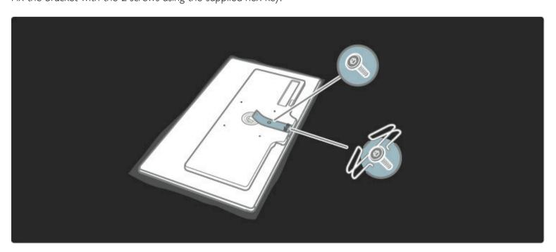
Position the bottom plate on the bracket as shown.
