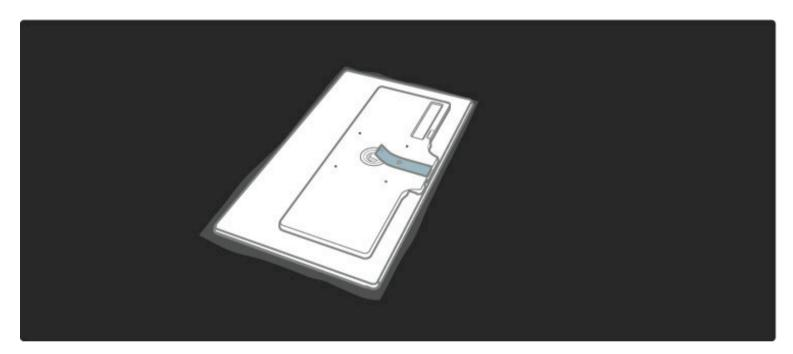
Fix the bracket with the 2 screws using the supplied hex key.
