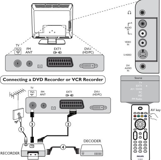
Connect the aerial cable ①. Use a good quality euroconnector cable ② to obtain the optimum picture quality. If your recorder does not have a euroconnector socket, the only connection possible is via the aerial cable ③. You will therefore need to tune in your video recorder's test signal and assign it programme number 0 or store the test signal under a programme between 90 and 99 (see Manual Store on page 6). See also the handbook of your recorder.
