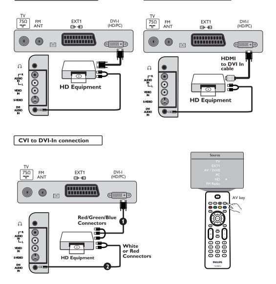
If you are using a High Definition equipment that can produce high definition signals, the TV can accept those signals by carrying out the connections below.
