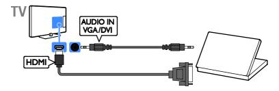
Connect the computer with a VGA cable and an audio cable to the TV.
