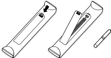
Insert the two R6-type batteries (supplied) making sure that they are the right way round.
