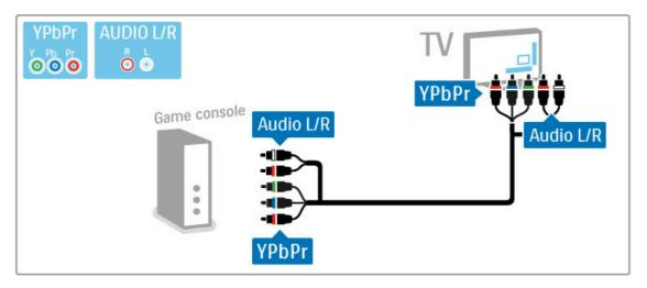
Or use Video and Audio L/R cables to connect the device to the  $\ensuremath{\mathsf{TV}}$
