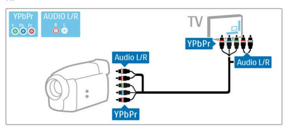
Or use Video and Audio L/R cables to connect the device to the  $\mathsf{TV}$
