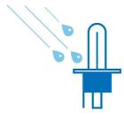
Only a burning bulb made of quartz glass (filament 2650°c, glass 800°c) can resist thermal shocks: if a drop of cold water touches
