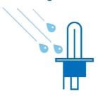
Only a burning bulb made of quartz glass (filament 2650°c, glass 800°c) can resist thermal shocks : such as, if a drop of cold water touches the hot bulb, when you drive through water with a broken headlight
