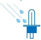
Only a burning bulb made of quartz glass (filament  $2650^{\circ}$ c, glass  $800^{\circ}$ c) can resist thermal shocks: such as, if a drop of cold water touches the hot bulb, when you drive through water with a broken headlight unit.
