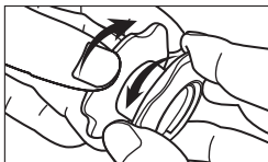
4. Unscrew the sensor cover by using the sensor tool
