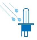
Only a burning bulb made of quartz glass (filament 2650°c, glass 800°c) can resist thermal shocks : such as, if a drop of cold water touches the hot bulb, when you drive through water with a broken headlight unit.
