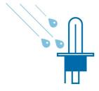
Only a burning bulb made of quartz glass (filament 2650°c, glass 800°c) can resist thermal shocks : such as, if a drop of cold water touches the hot bulb, when you drive through water with a broken headlight unit.
