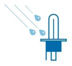
Only a burning bulb made of quartz glass (filament 2650°C, glass 800°C) can resist thermal shocks, such as when a drop of cold water touches the hot bulb, which can happen when you drive through water with a broken headlight unit. ^Application varies per bulb type
