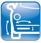
The mounting range of the modules has increased to  $\pm$ -40 degrees horizontally,  $\pm$ -2
