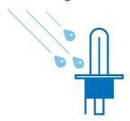
Only a burning bulb made of quartz glass (filament 2650°c, glass 800°c) can resist thermal shocks : such as, if a drop of cold water touches the hot bulb, when you drive through water with a broken headlight
