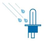
Only a burning bulb made of quartz glass (filament 2650°c, glass 800°c) can resist thermal shocks: if a drop of cold water touches the hot bulb, which can happen when you drive through water with a broken headlight unit.
