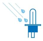
Only a burning bulb made of quartz glass (filament 2650°c, glass 800°c) can resist thermal shocks : such
