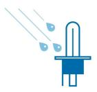
Only a burning bulb made of quartz glass (filament 2650°c, glass 800°c) can resist thermal shocks: if a drop of cold water touches the hot bulb, which can happen when you drive through water with a broken headlight unit.
