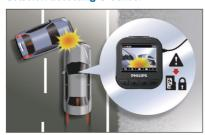
The Philips ADR620 comes equipped with a 3-axis G-sensor module, which detects movement and triggers an emergency recording mode. In the event of a collision that exceeds a certain force threshold, the device will lock that video clip to prevent it being overwritten. This important video is then safely secured on a durable memory card. R85
