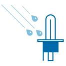
Only a burning bulb made of quartz glass (filament 2650°c, glass 800°c) can resist thermal shocks: if a drop of cold water touches the hot bulb, which can happen when you drive through water with a broken headlight unit.
