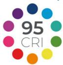
The higher the Color Rendering Index (CRI3), the easier it is to perform a quick and accurate inspection of car bodywork. You can inspect your paint, polish, clean, or prep zone as if you were working outdoors on a bright sunny day. Lamps with a low CRI value cause some colors to appear unnatural. Light sources with a CRI of 90 or above will let you easily and quickly spot color differences such as paint scratches.
