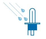
Only a burning bulb made of quartz glass (filament  $2650^{\circ}$ c, glass  $800^{\circ}$ c) can resist thermal shocks : if a drop of cold water touches the hot bulb, which can happen when you drive through water with a broken headlight unit.
