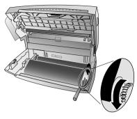
11 Close the device. Insert the paper tray in the opening provided for it behind the paper feeder. Insert paper
