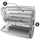
**5** Clean the feed roller (**A**) and the underside of the support pad of the feeder roller (B) with a soft, lint-free cloth moistened with cleaning alcoho 1 (96 percent). Rotate the feed roller; You must clean the entire roller.
