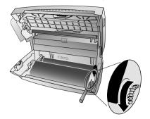
**5** Close the device. Insert the paper tray in the opening provided for it behind the paper feeder. Insert paper again.
