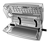
Remove both the rolls from the device. The used ink film cannot be reused.
