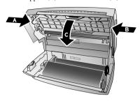
4 Carefully pull the document to the front or to the back out of the device.
