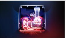
Our all-in-one Screeneo S Collection projectors are designed to dissipate heat throught the aluminum side grids along with a state-of-the art ultra low noise fan.
