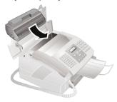
7 Close the cover. Make sure that the cover snaps securely into position on both sides.
