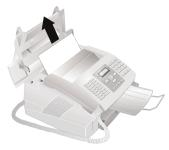
In case of a paper jam, do not forcefully remove the paper, but rather pull it gently out of the device and throw it away carefully. It is possible that the toner may not be completely set on the printout, and toner dust could be released into the air. Do not inhale the released toner dust. Remove the toner dust from clothing or objects with cold water; hot water would only cause the toner to set.
