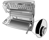
7 Close the device. Insert the paper tray in the opening provided for it behind the paper feeder. Insert paper
