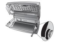
7 Close the device. Insert the paper tray in the opening provided for it behind the paper feeder. Insert paper again.
