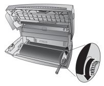
II Close the device. Insert the paper tray in the opening provided for it behind the paper feeder. Insert paper again.
