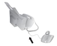
We recommend direct connection to the device because this allows the fax switch to function optimally and to control the additional devices.
