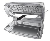
**4** Turn the blue gear wheel forward to tension the ink film. The ink film must not have any creases.
