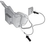
If you connect your device as extension to a telephone system, you must set it for working as an extension (also see Chapter "Telephone connections and additional devices, page 21).
