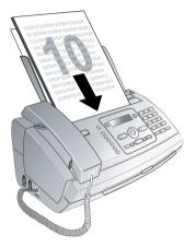
2 Set the desired resolution. You can choose between RESOL.: STANDARD (for documents without special features), RESOL.: FINE (for texts with small print or drawings) and RESOL.: PHOTO (for photos). Press I. The configured resolution appears on the display. Press II again to change the resolution.
