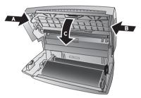
**4** Carefully pull the document to the front or to the back out of the device.
