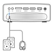
2 After connecting the speakers or headphones, press the volume control buttons on a remote control to adjust the volume to the desired level
