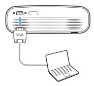
2 Adjust your computer's screen resolution to the correct setting and switch the VGA signal to an external monitor. The following resolutions are supported:
