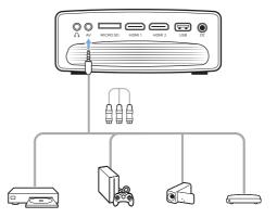
2 Press on the projector remote control to display the input source list, and then select AV.
