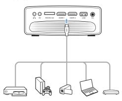
2 Press → on the projector remote control to bring up the input source list, and then select HDMI1 or HDMI2.
