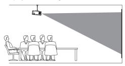
2 To adjust projection to the correct position, press (○=)/-(-) on the remote control to access the settings menu and navigate to Projection Direction - Front Ceiling.
