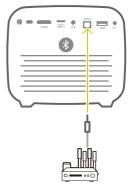
2 To output audio to the external device, make sure external speaker output is activated. Press (○三)/+□ to access the settings menu and select Audio Output -Optical.
