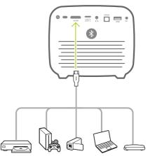
2 The projector automatically switches to HDMI input when HDMI connection is made. The projection screen shows images.
