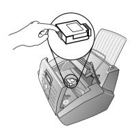
4 Remove the cartridge by pulling it up diagonally forward and taking it out.
