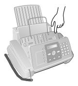
**3** Press the lock in the centre of the holder towards the front and lift the cartridge.
