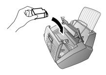
**7** Press the cartridge down until it snaps into place.
