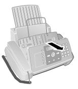
2 Open the cartridge compartment by pressing on the upper right corner of the document holder (arrow) and then carefully lifting it backwards. Click the document holder completely in place.
