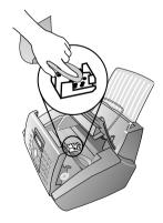
5 Insert the cartridge and close the device.
