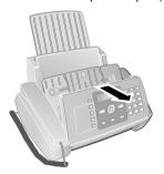
2 Open the cartridge compartment by pressing on the upper right corner of the document holder (arrow) and then carefully lifting it backwards. Click the document holder completely in place.
