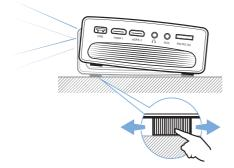
3 To adjust image focus, turn the focus knob on the top of the projector.
