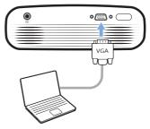
On your computer, adjust the screen resolution of the computer to the correct setting and switch the VGA signal to an external monitor. The following resolutions are supported:
