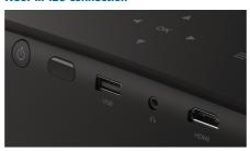
Connect any media device: set-top boxes, computers, game consoles and streaming boxes such as Fire Stick or Apple TV thanks to its built-in USB, HDMI. Enough of wires! Connect your smart dongles (Amazon Fire Sticks, Roku...) to the USB power out (5V2A) and get rid of an external adapter.
