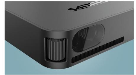
A super slim 18mm projector featuring premium dark grey metal finish with glass protection lens. The cabinet design has been engineered to create a passive heat dissipation. Moreover, both the cabinet vent system and speaker moulding have been designed for improved rigidity.
