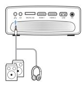
2 After connecting the speakers or headphones, press the volume control buttons on a remote control to adjust the volume to the desired level.
