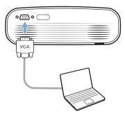
2 Adjust your computer's screen resolution to the correct setting and switch the VGA signal to an external monitor. The following resolutions are supported:
