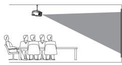
2 To adjust projection to the correct position, press ♠, and select Settings - Advanced Settings - Projection Location - Front Ceiling.
