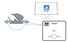
Or to adjust image shape, press ♠, and select Settings - Advanced Settings - V. Keystone, then press ◄/▶ on the remote control to adjust the screen position.
